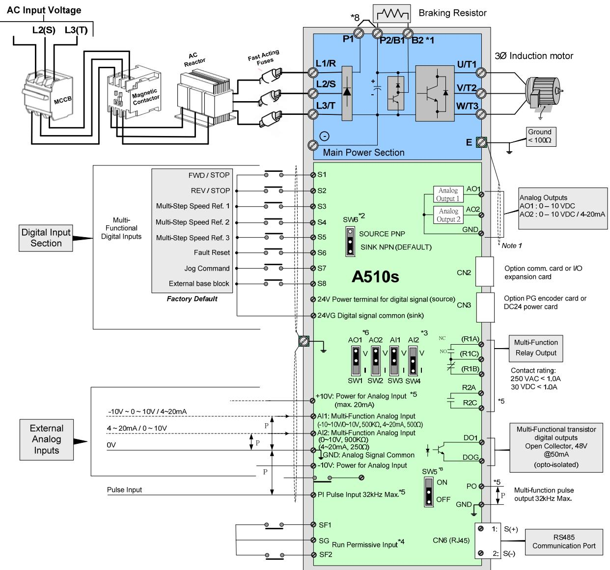
\*9: Only the model 200V 3~40HP and 400V 5~75HP provide P1 and P2 terminal, for external DCL connected. P1 and P2 are short-circuited before shipping out from the factory.
